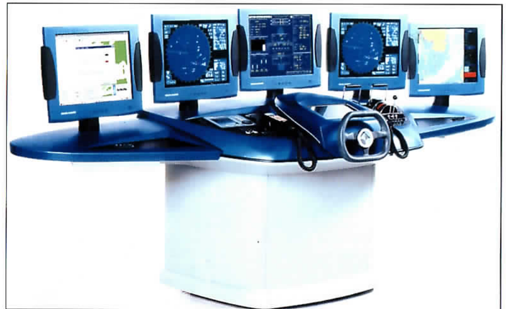
Designer Jon Bannenberg specified flat screen LCD monitors that could be tiled vertically and horizontally to give a head-on view from anywhere on the bridge
